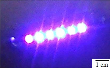
Figure 8.2: Wearable electronics: body as a primary substrate for active device. A. Electronics with active LEDs and interconnects directly mounted onto the skin. Device is not in operation ( a 1 ) and in operation ( a 2 ). The left images ( i ) show the electronics in normal condition and the right images ( ii ) show the device under mechanical stress.
