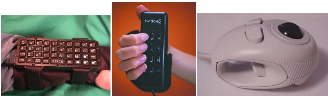
Figure 1: Derivatives of traditional user interfaces. From left to right: L3 Systems WristPC attachable keyboard, Handykey Twiddler, Finger Trackball
