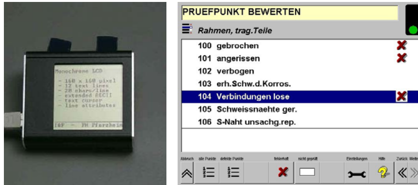
Figure 2: Examples for small display (12 lines, 20 char.) and GUI design with traffic light symbol
