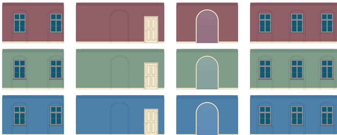
Fig 5: Coloured Architecture: automatically generated wall and floor/ceiling elevations using colour profiling from CAAD model (Wielandgut Osmanstedt, Ausführungsprojekt, 2004 © nitschke-donath weimar)
