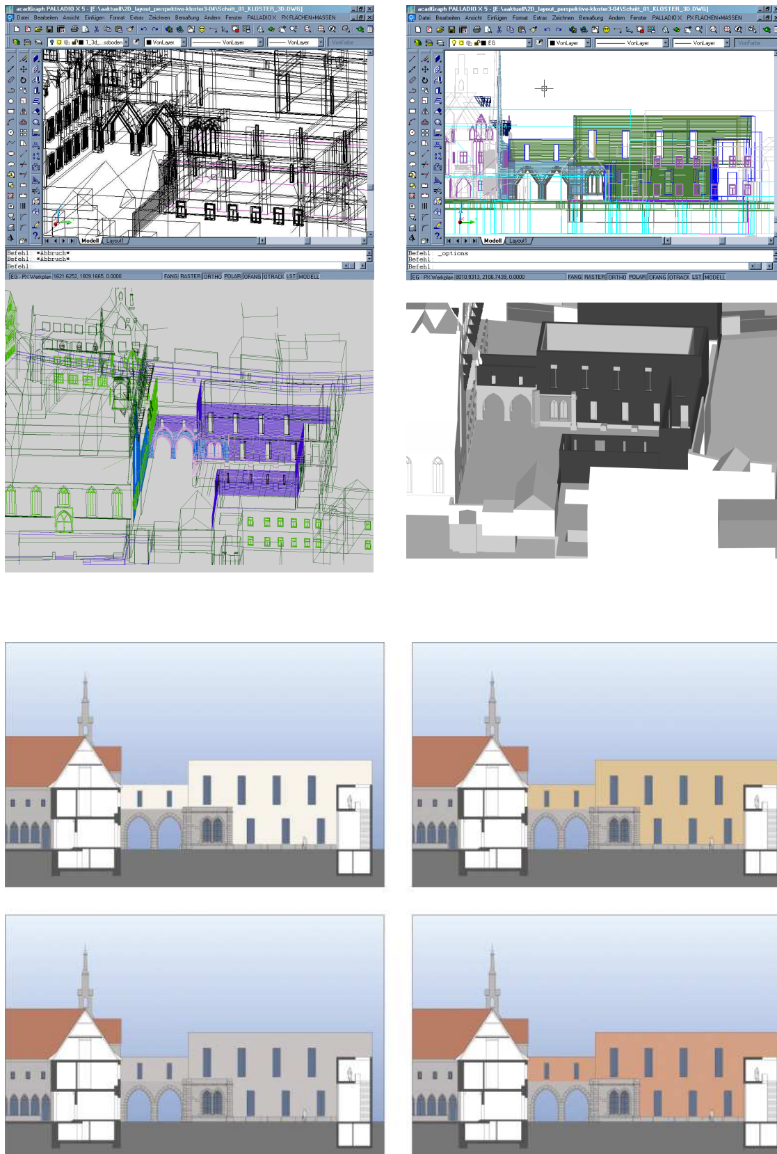
Fig. 3 Coloured Architecture: comparison of colour scheme variants using 2D-views of a CAAD building model (Augustiner-Kloster Erfurt, Competition, 2004 © nitschke-donath architekten)
