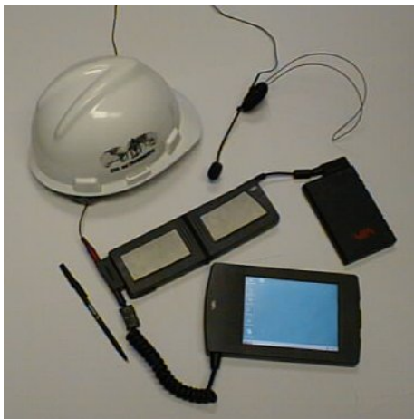
b) MIA Hardware: 180 MHz ViA System with noise canceling microphone
