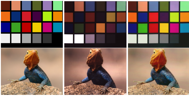
Figure 4: Color reconstruction of Macbeth samples (top) and digital image (bottom) developed on photographic paper with a Kodak System 88 digital lab system. The original (left), rectified camera image of photo without (center) and with (right) reconstructed colors. The reconstructions show a 4% chrominance deviation to original in CIE L^*a^*b^* space.
