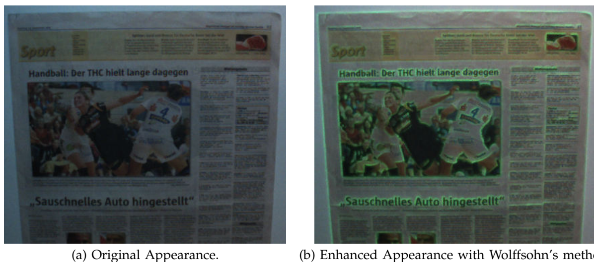
Fig. 4. Enhancement Result by Wolffsohn's Method: The picture in the news paper contains complex background and its visibility not good for low vision (a). The edge is detected with Prewitt filter and overlaid onto green illumination with projector camera feedback (b). The edge line in the picture is easily understandable and it gives a benefit for low vision.
