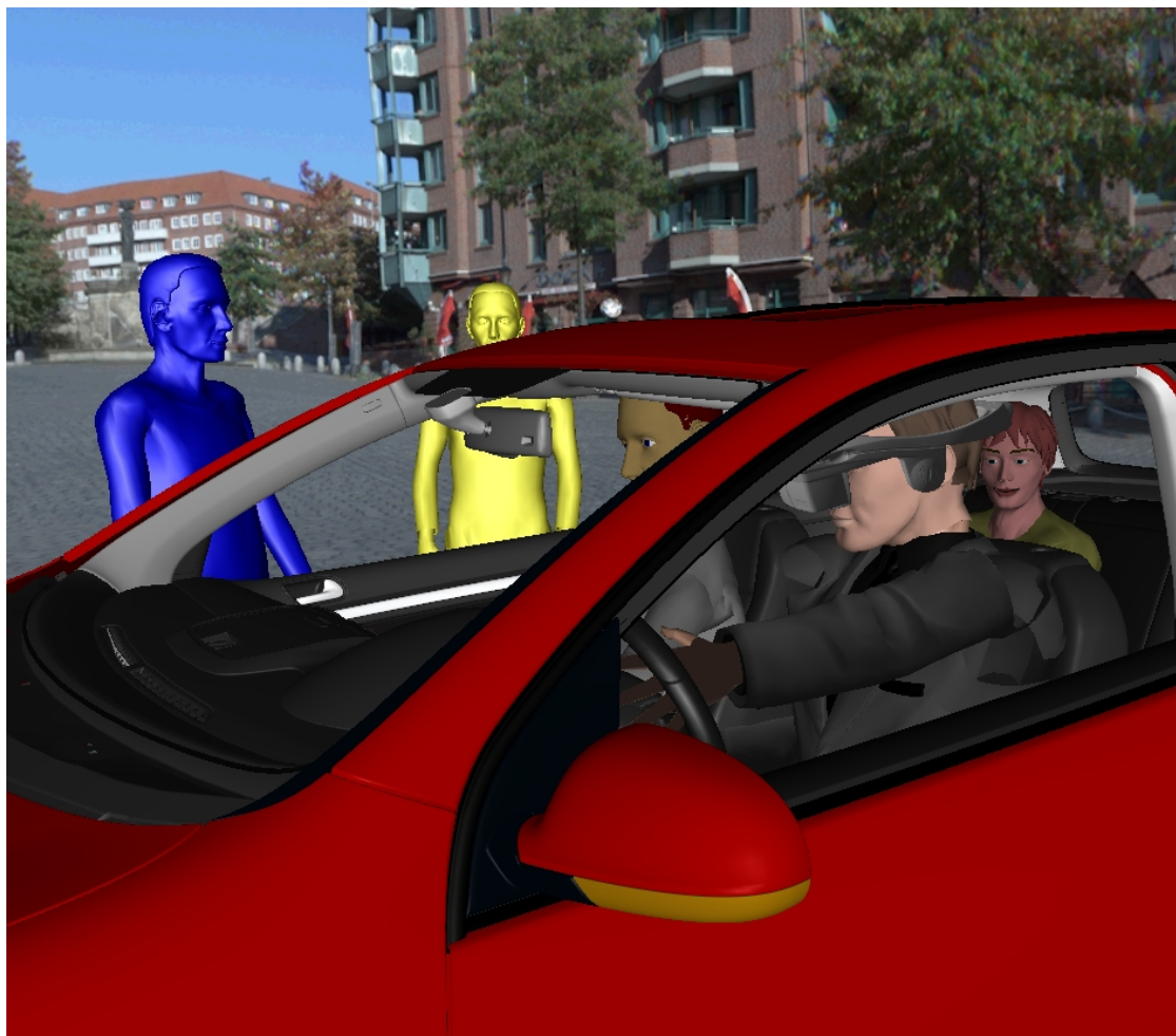
Figure 7.1: Additional users participating in a virtual seating buck session provided with an individual stereoscopic view and visible to their colleagues via their avatars.
