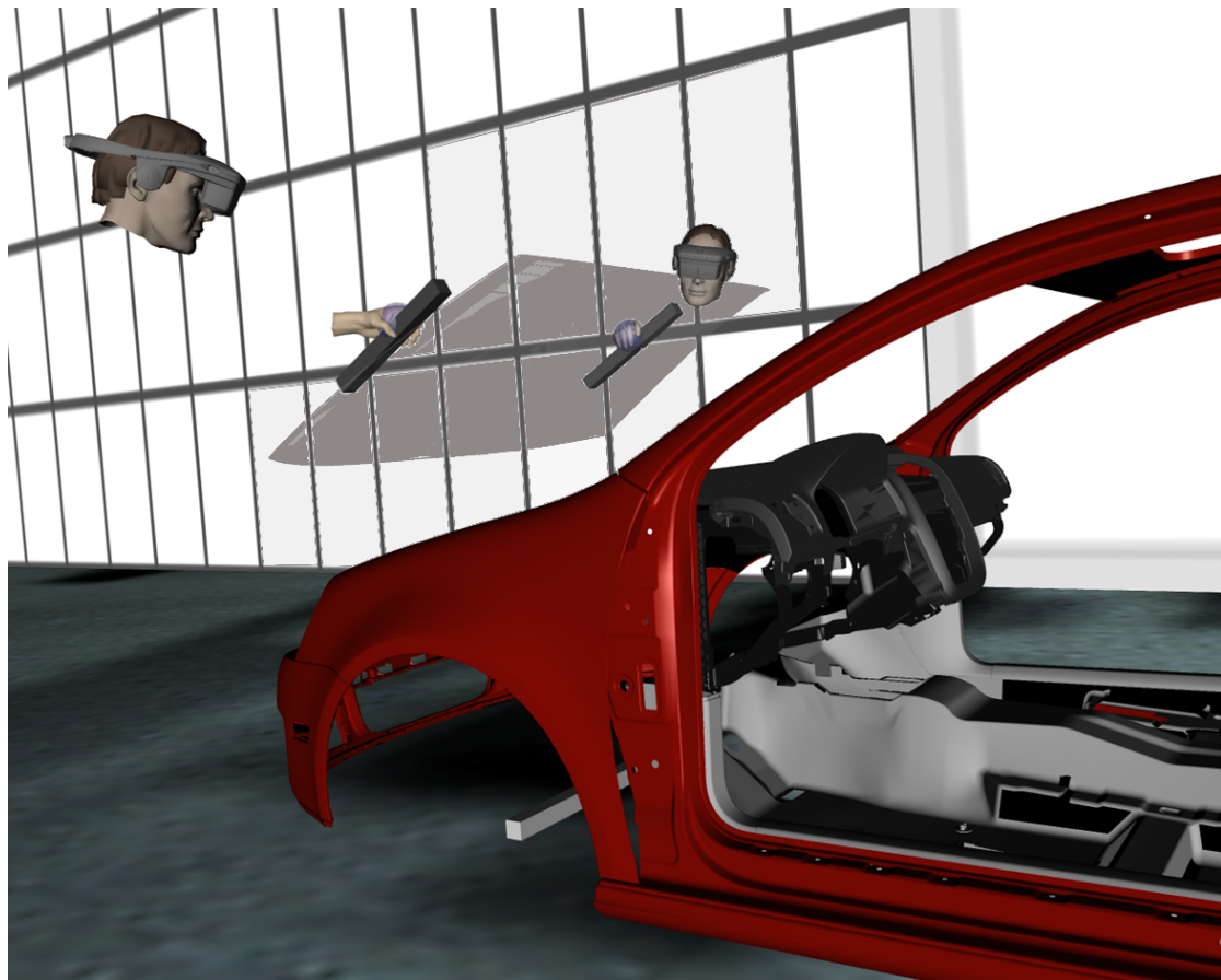
Figure 5.4: The basic avatars, the virtual windshield with its handles including small spheres representing the grab positions, the car and an assembly hall as background were composed in the virtual environment.
