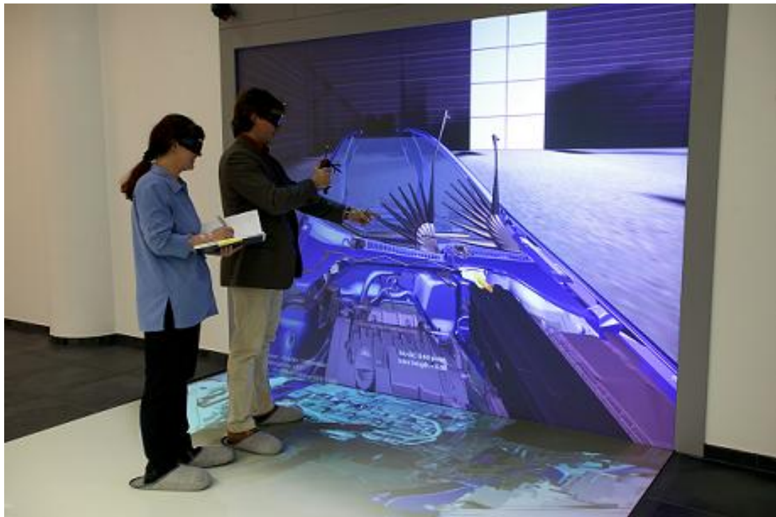
Figure 1.3: One tracked user and one non-tracked user in front of an L-shaped projection screen.
