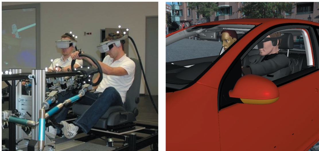
Figure 6.1: The two-user seating buck scenario. The image on the left side shows the hardware setup. The right side shows the same perspective for the virtual car model including the two avatars.
