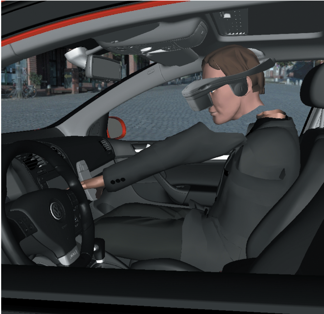
Figure 6.7: When the user leans forward and stretches his arm in order to reach the navigation device, the simplified body model produces gaps between the moving body parts and the fixed torso.
