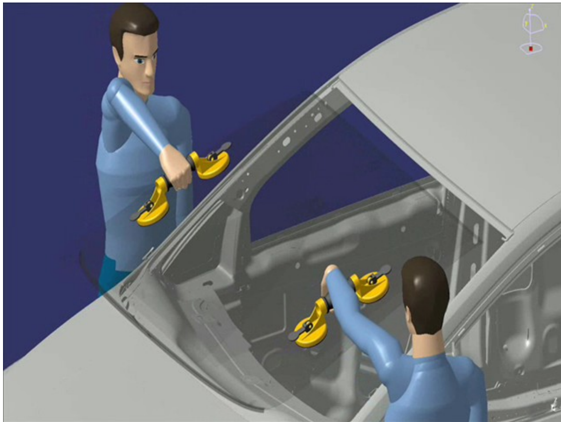
Figure 5.2: Snapshot from the video showing the process animation of the windshield assembly task.
