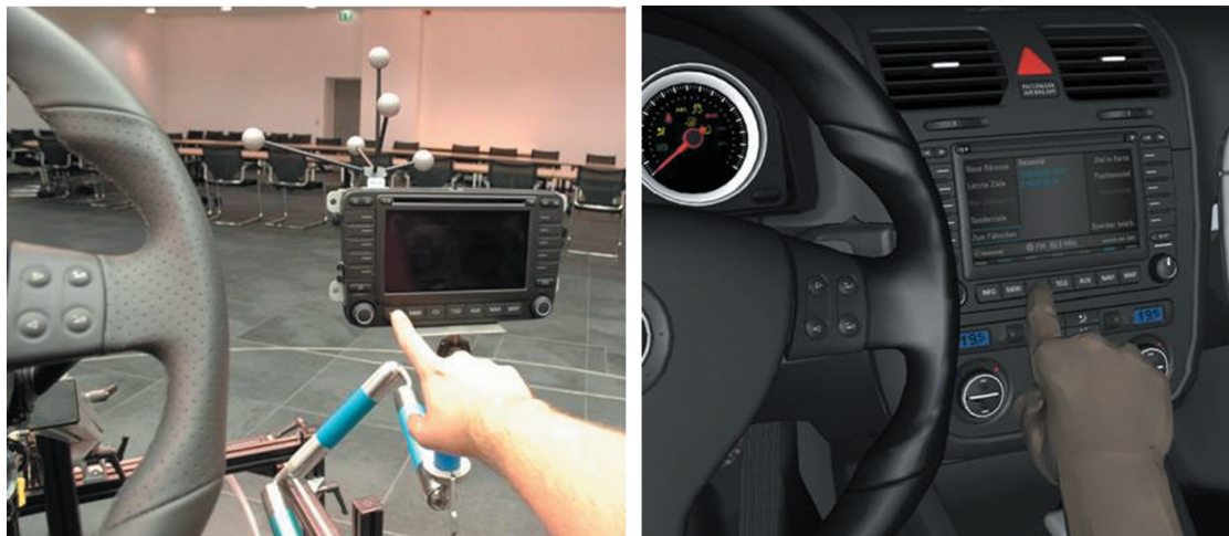
Figure 6.3: On the left side the navigation device panel mounted on an arm of the flexi-holder is shown and on the right side the corresponding virtual image through the driver's HMD.
