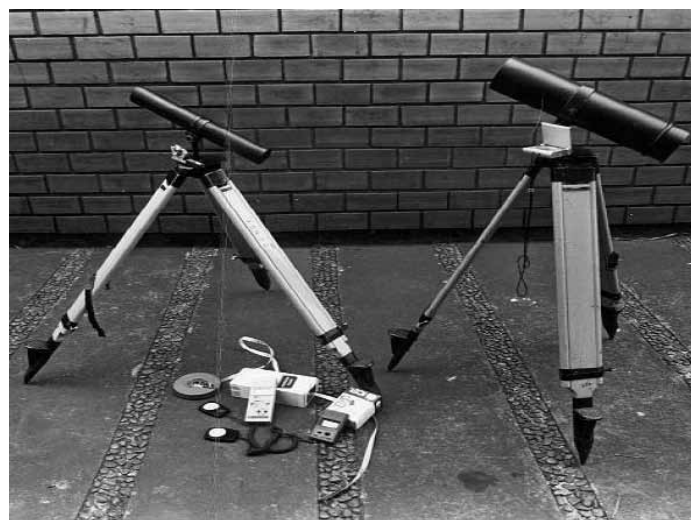
Fig 4.16: Tube Luximeters used by Pietrobon (1999) (left) Set of pyranometers used by Ali-Toudert (2005) in Freiburg to measure mean radiant temperature.
