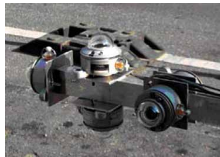
Fig 4.16: Tube Luximeters used by Pietrobon (1999) (left) Set of pyranometers used by Ali-Toudert (2005) in Freiburg to measure mean radiant temperature.
