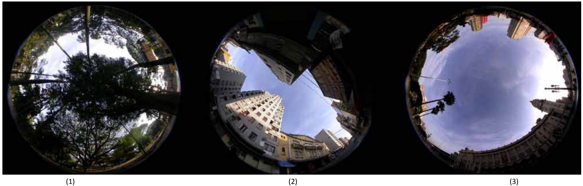
Figure 3. Hemispheric pictures of the sky view taken with a Nikon 4500 equipped with a 180° fish eye lens for park (1), canyon (2) and open square (3). Source: LABAUT
