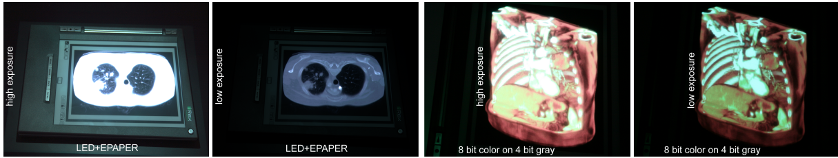
Figure 5: Contrast enhanced ePaper (captured with different exposures and color modulated).
