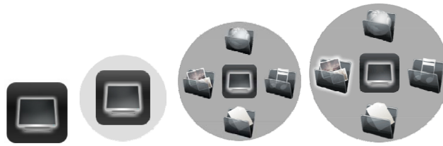
Figure 13: The Radial Saccade Pie Menu. Upon gaze entering the component a opaque ellipse expands from underneath the button. Four icons appears on the ellipse. A fixation starts the activation process which is indicated by a glowing border. Both the expansion time and activation time can be configured. The number of icons used is optional between 1-4 (image courtesy of Martin Tall) [76].
