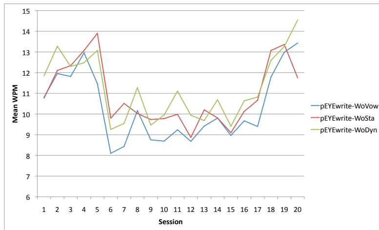
Figure 46: Word per minutes achieved with the bigram text entry methods combined with word prediction on each session.
