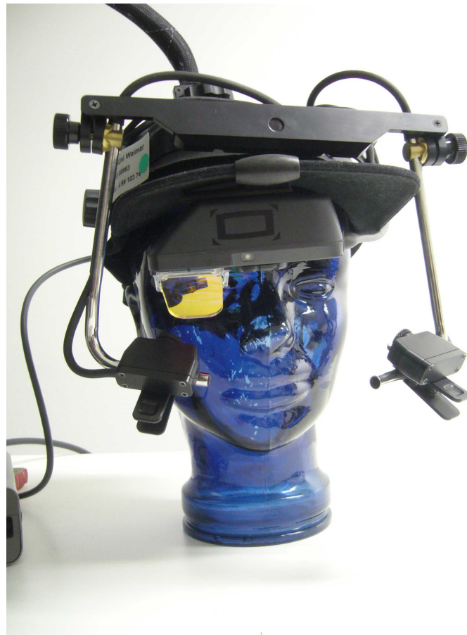
Figure 57: Set-up of the OST-HMD with the EyeTracker.
