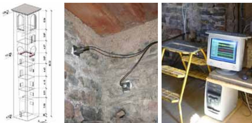
Figure 6 — General arrangement of the dynamic monitoring system
