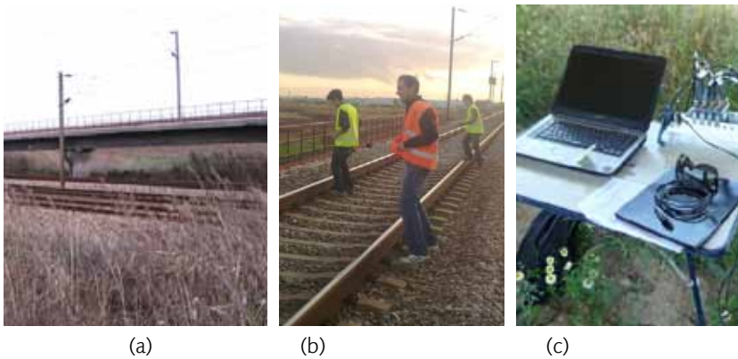
Figure 3 — Ambient vibration test: (a) instrumented spans; (b) external excitation; (c) acquisition system
