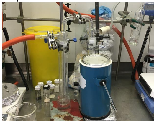
Figure 4.12. Images demonstrating the apparatus set-up used to generate \text{SO}_2\text{ClF} .
