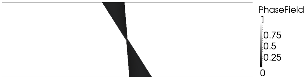
Figure 4.26: Evolution of the crack front in the beam seen from the top, the maximum and the minimum of phase field, i.e. v = 1 and v = 0 are shown.
