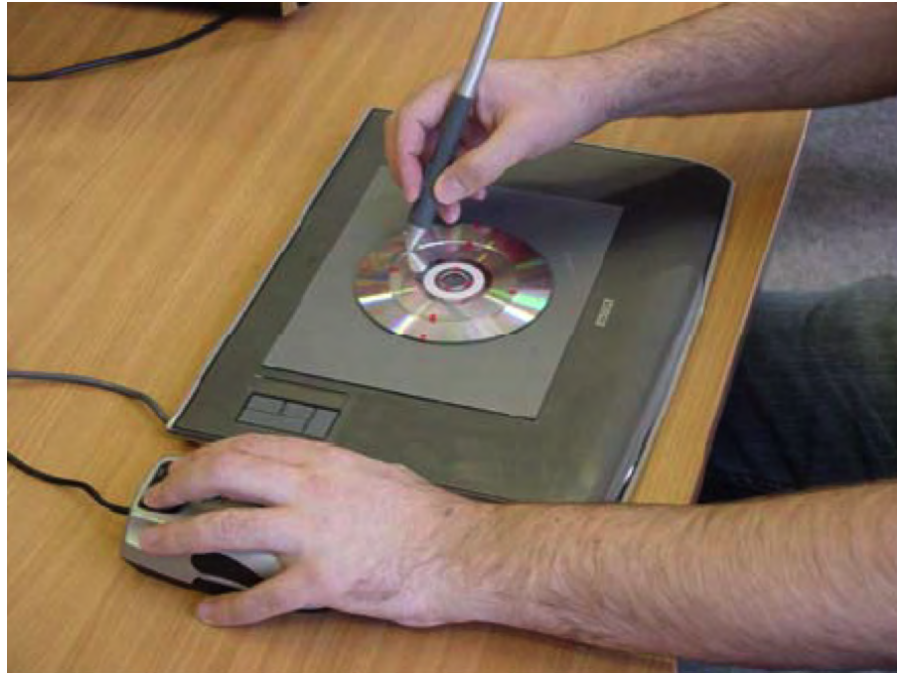
Figure 19: Tac-tile system. Graphics tablet augmented with a tangible pie chart relief, with dynamic tactile display [302]
