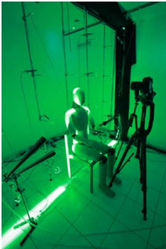
Fig. 3. Climate chamber with thermal manikin. Visible are also the diffusers of the particle streak tracking and the flow field illuminated by LEDs. In the background, several temperature and air velocity sensors are installed.
