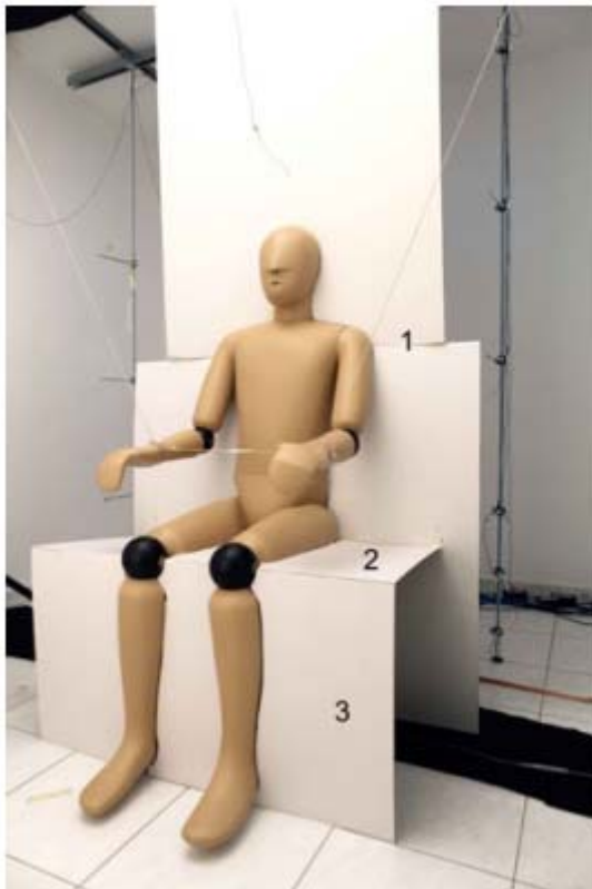
Fig. 4. Work plane made of cardboard surrounding the thermal manikin
