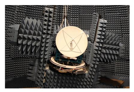
Figure 7.1: The antenna under test while being mounted on the motion emulator and tested at the Fraunhofer Facility for Over-the-air Research and Testing (FORTE).
