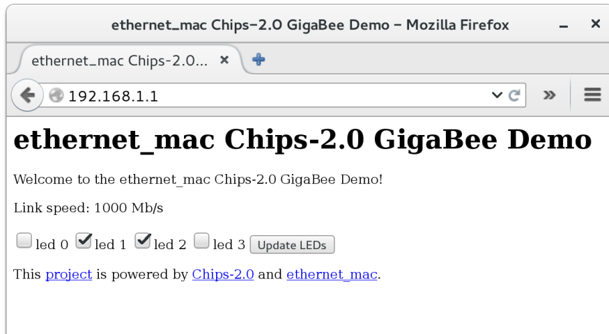
Figure 6.1: Index page of the modified Chips webserver demo project using the MAC sub-layer presented in this thesis
