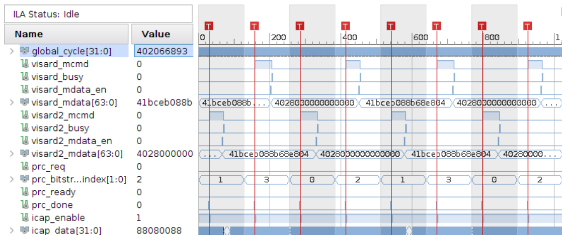
Figure 5.5: Recorded waveform showing parallel reconfiguration and calculation of two ViSARD cores working in practice. All numbers captured on buses are shown in hexadecimal notation except for global_cycle . The logic analyzer core was set to trigger on visard_mcmd or visard2_mcmd high (indicated by red vertical lines). Other ILA settings: 8 windows 128 samples deep each, trigger position in window at 30. Description of signals in Table 5.1 (prefix visard_ indicates the first, prefix visard2_ the second ViSARD core).
