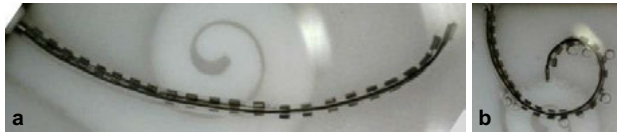
Figure 2: (a) Banana-shaped configuration of the electrode array at 23°C. (b) Final shape.
