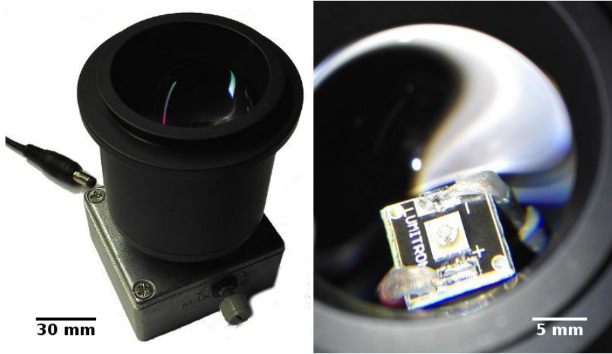
Figure 32: Developed high power UV-source using a NCSU276A LED (Nichia Corp., Japan) for in-house hard lithographic production of microchannel structures in SU-8, boxed and equipped with a \varnothing 75 mm collimation lens (Thorlabs) to expose silicon wafers of three inch diameter.
