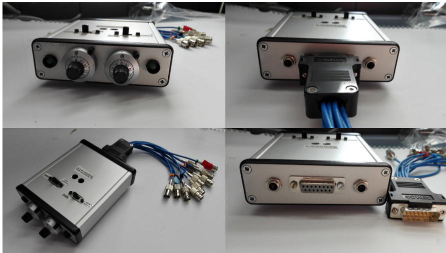
Figure 28: Final dual Schmitt trigger setup with modular D-sub connector interface.
