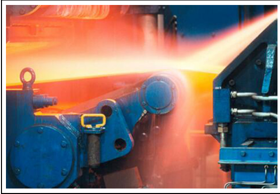
Figure 3. Looper system between rolling stands.
