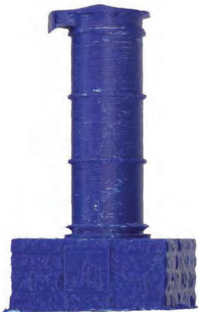
FIGURE 5. The Löbejün monument printed on a Dimension 1200es 3D printer from Stratasys. The final print was 19 cm high with a 10 × 10 cm base.
