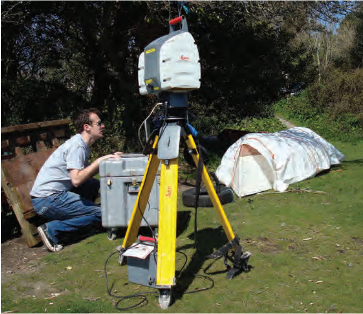
Figure 1. The Leica HDS3000 scanner used in our case study. This scanner is a time-of-flight, mid-range laser scanner with a built-in mechanical accuracy of \pm 5 mm, a 360-degree horizontal scan window, and a 270-degree vertical scan window.
