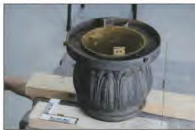
ImageMeter takes the x and y coordinates in a photograph and uses them for vector modelling
