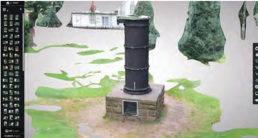
FIGURE 4. 3D scene of the Löbejün monument in Photo. The scene represents a triangular mesh of 5.63 million triangles. Users can view a generated mesh at reduced resolution before exporting it as a .rcm, .obj, .fbx, .rcs, or .ipm file.
