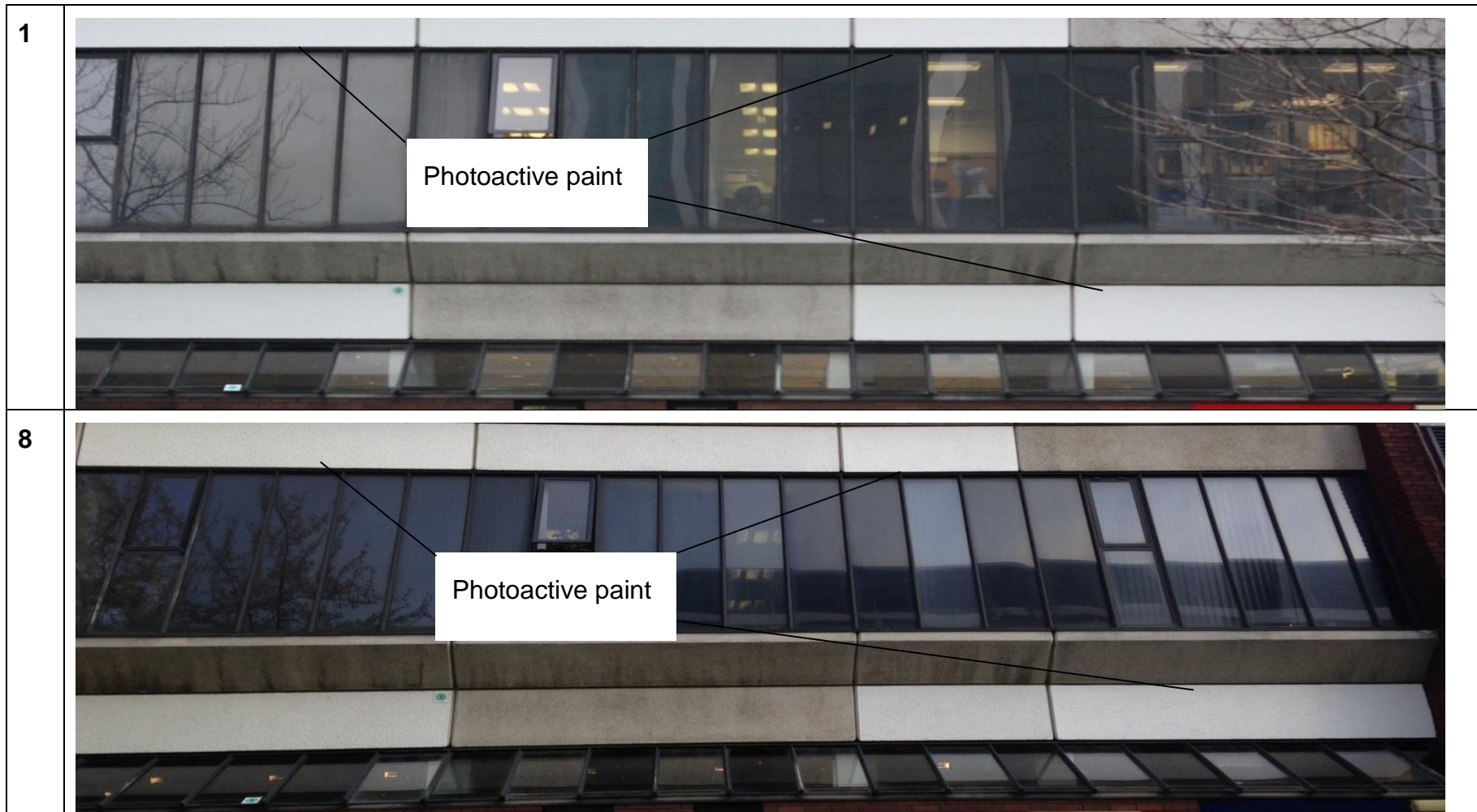
Figure 94: Photographs of the concrete panels after one month and after eight months. The panels treated with photocatalytic paint are labelled. The month is displayed on the left. The photocatalytic panels appear similar to the inactive painted panels at one month, but appear cleaner after eight months.
