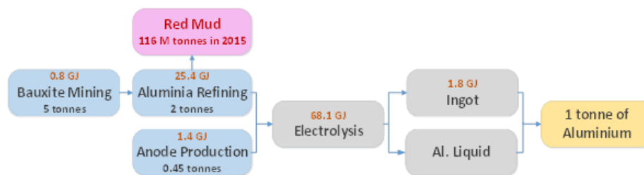
Figure 2. Primary aluminum production steps with associated energy content for producing one ton of material.
