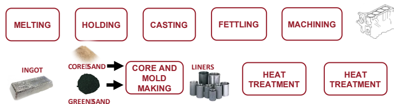
Figure 7. Process flow for Al-alloy engine block manufacturing.
