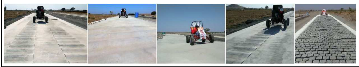
Figure 4. Test tracks used, left to right: washboard, herringbone, chassis-twist, one-sided washboard, and Belgian pave.
