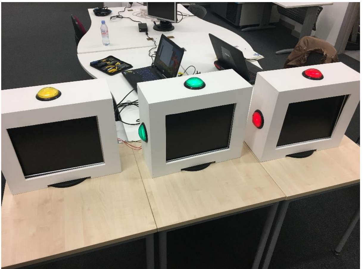
Figure 111 Assembly monitors encased in the cabinets
