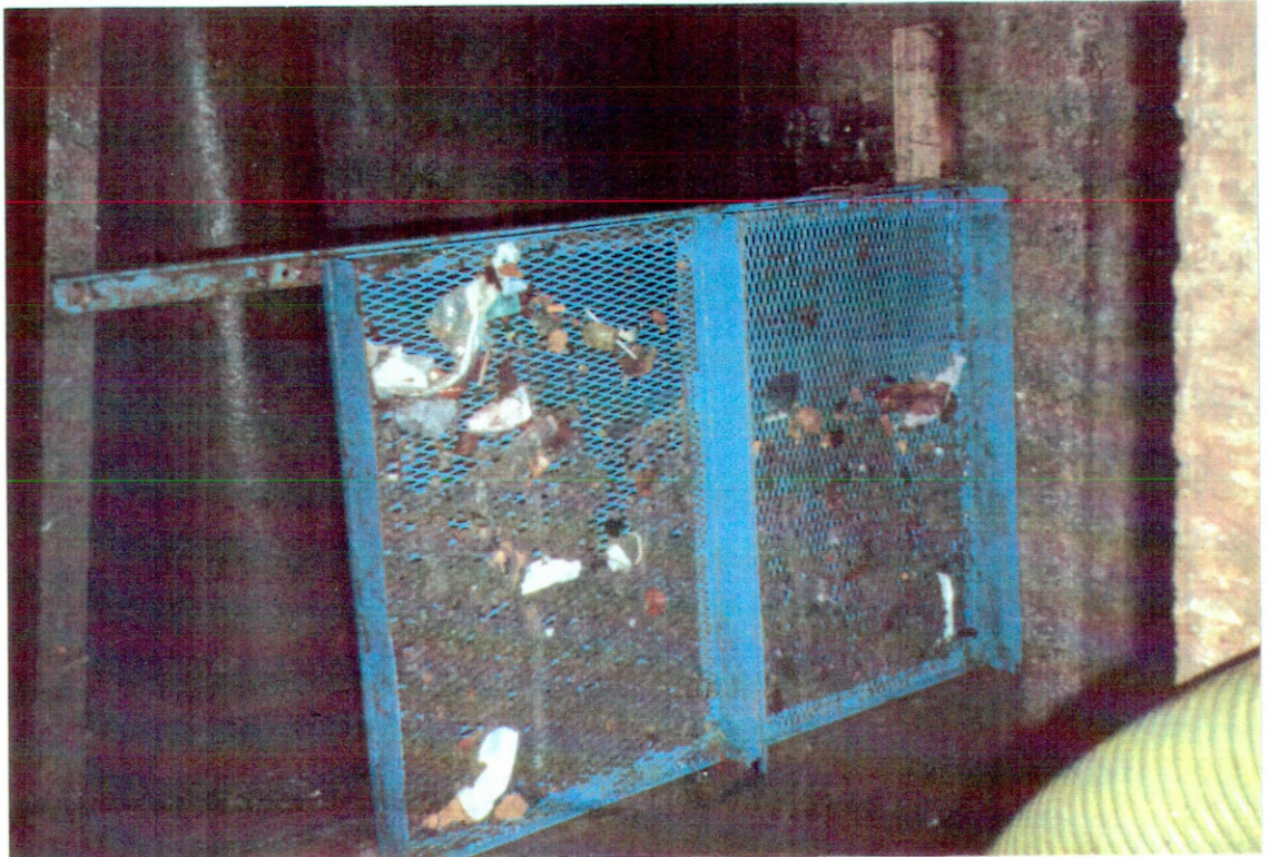
Plate 5.2 Trash Trap Event 8 on 25/11/90 Broomhead Blinding 50% Mass Collected 47.9g Number of Visible Solids = 12
