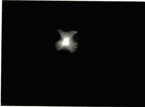
Fig. 6.6. The intensity correlation result obtained with conventional holographic recording in BSO (O/R = 1/2 in average).
