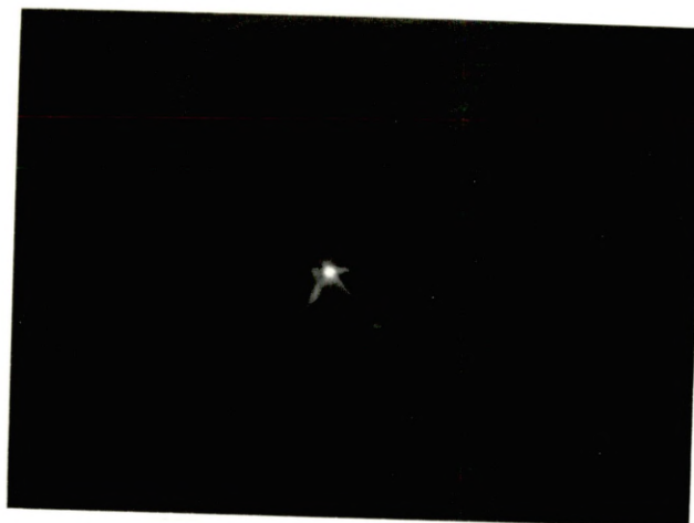
Fig. 6.8. The intensity correlation result obtained with nonlinear holographic recording in BSO (O/R = 10/1) in average).
