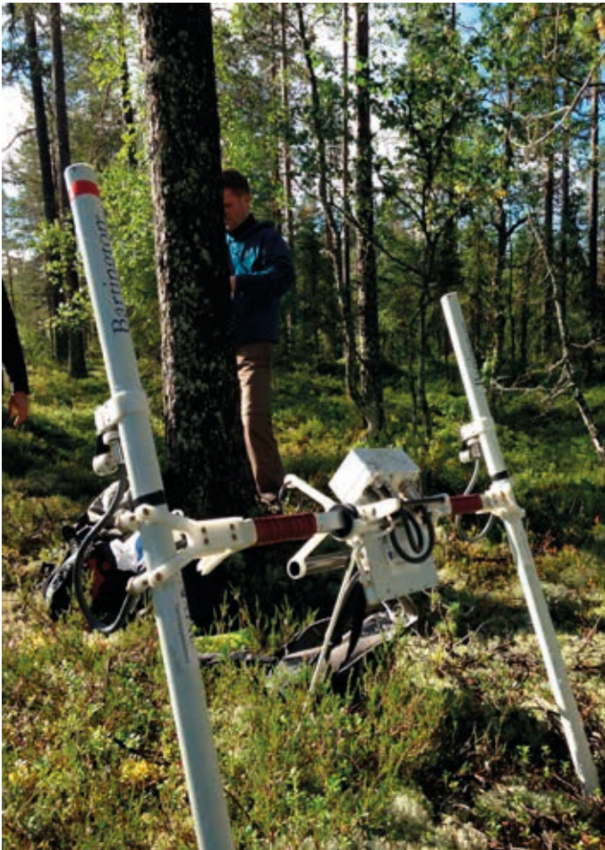
Figure 2: The dual sensor Bartington Grad 601 gradiometer used in the surveys presented in this article
