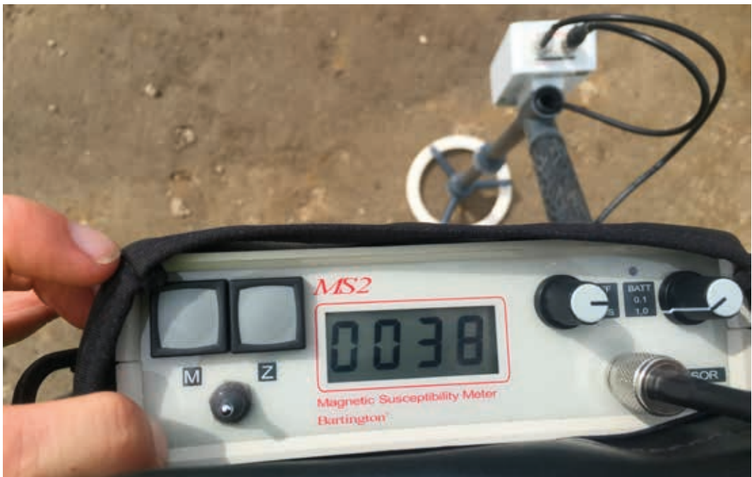
Figure 1. Measuring magnetic susceptibility with the Bartington MS2 Magnetic susceptibility meter
