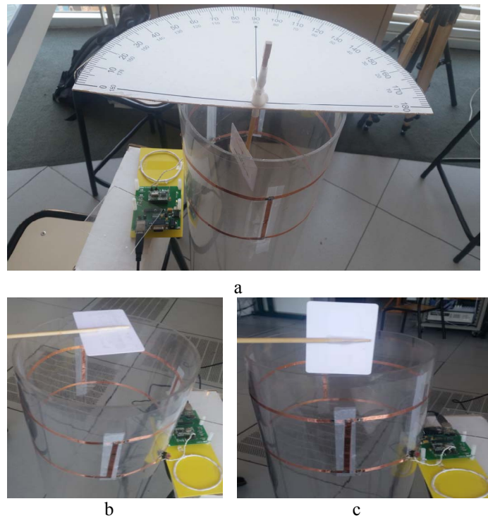
Fig.7. Realized 3D design with the tag inside the tube (a), parallel to the tube (b) and perpendicular to the edges of the tube (c)
