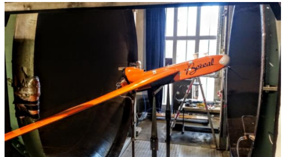
Figure 10: BOREAL during the wind tunnel test
