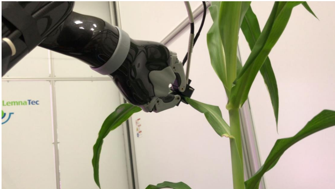
Fig. 2.16. The robotic manipulator grasps the leaf to take measurements
