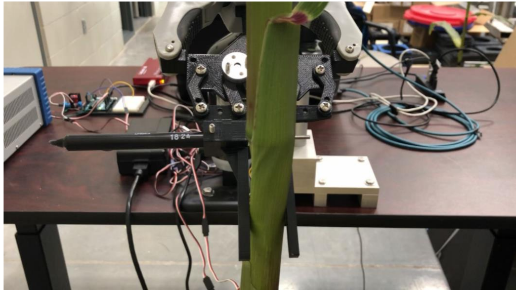
Fig. 3.11. The robotic manipulator grasped the stem to take its diameter measurement
