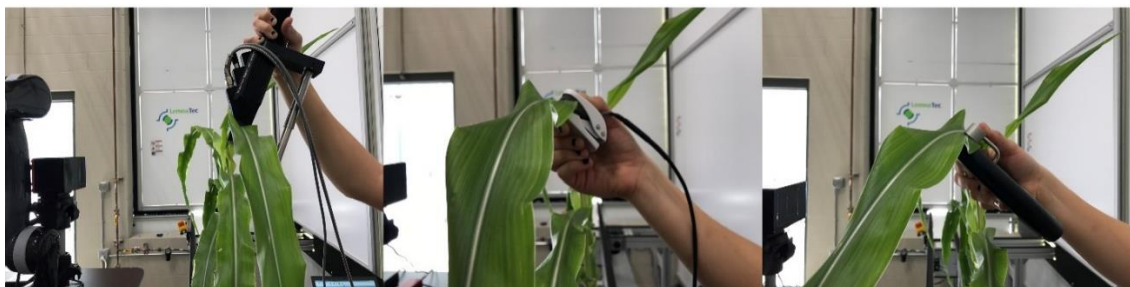
Fig. 2.20. Ground-truth measurements by a researcher: leaf reflectance spectrum (left), leaf temperature (middle), and leaf chlorophyll content (right).
