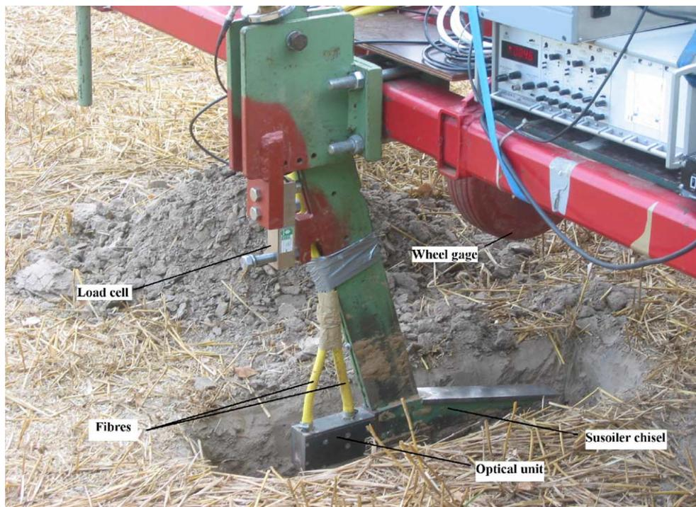
**Figure 1.6. Subsoiler-optical unit set up developed by Mouazen, De Baerdemaeker, and Ramon (2005).**
