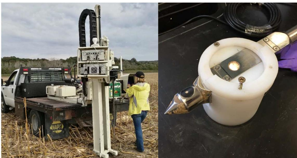
**Figure 1.14. Left: Veris<sup>®</sup> P4000 used by Veum, Parker, Sudduth, and Holan (2018) in the field. Right: close-up view of P4000 probe tip adapted for acquiring air dry spectra.**
