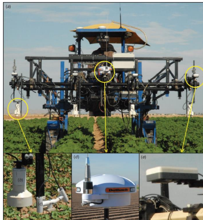
Figure 1.2. The Maricopa phenotyping system: (a) front view; (b) the sonar proximity sensor; (c) the infrared radiometer; (d) the GPS receiver; (e) the multispectral crop canopy sensor (Andrade-Sanchez et al. 2014).
