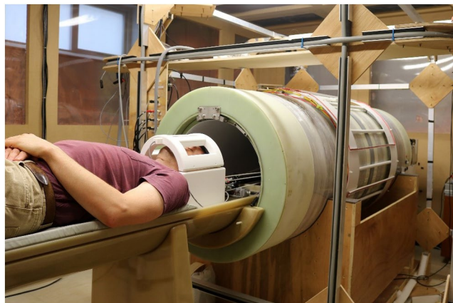
Figure 1. Front view of the FFC-MRI scanner presented here. The scanner has a bore of 50 cm and is surrounded by three pairs of Helmholtz coils for the correction of the Earth's magnetic field (square section coils visible around the scanner). A volunteer can be seen on the patient table, his head within a birdcage head coil, prior to insertion into the bore of the main magnet.
