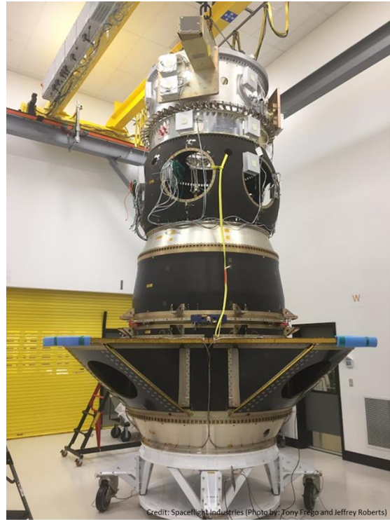
Figure 7: Launch Adapters Used in the Full SSO-A Launch Stack
