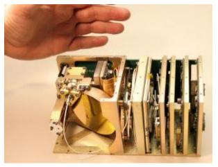
Figure 2: Fibertek's Compact Laser Communications Terminal.
