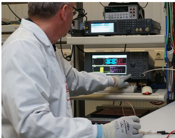
Figure 4: XLink RF Performance Testing
