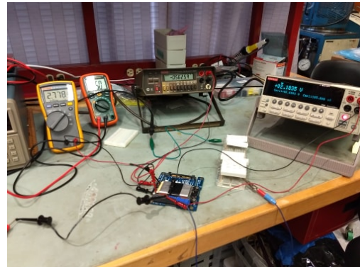
Figure 8: Remote Battery Board under Test
