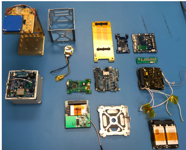
Figure 12: Major satellite bus components prepared before integration
