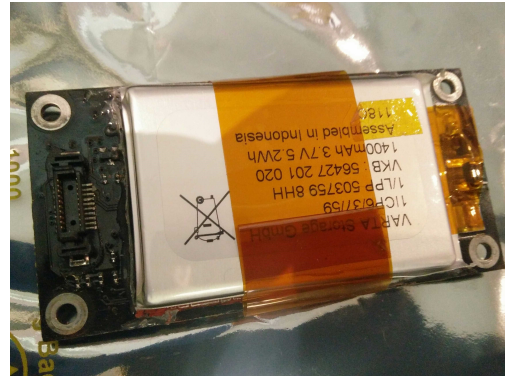
Figure 11: Remote Battery board ready for integration
