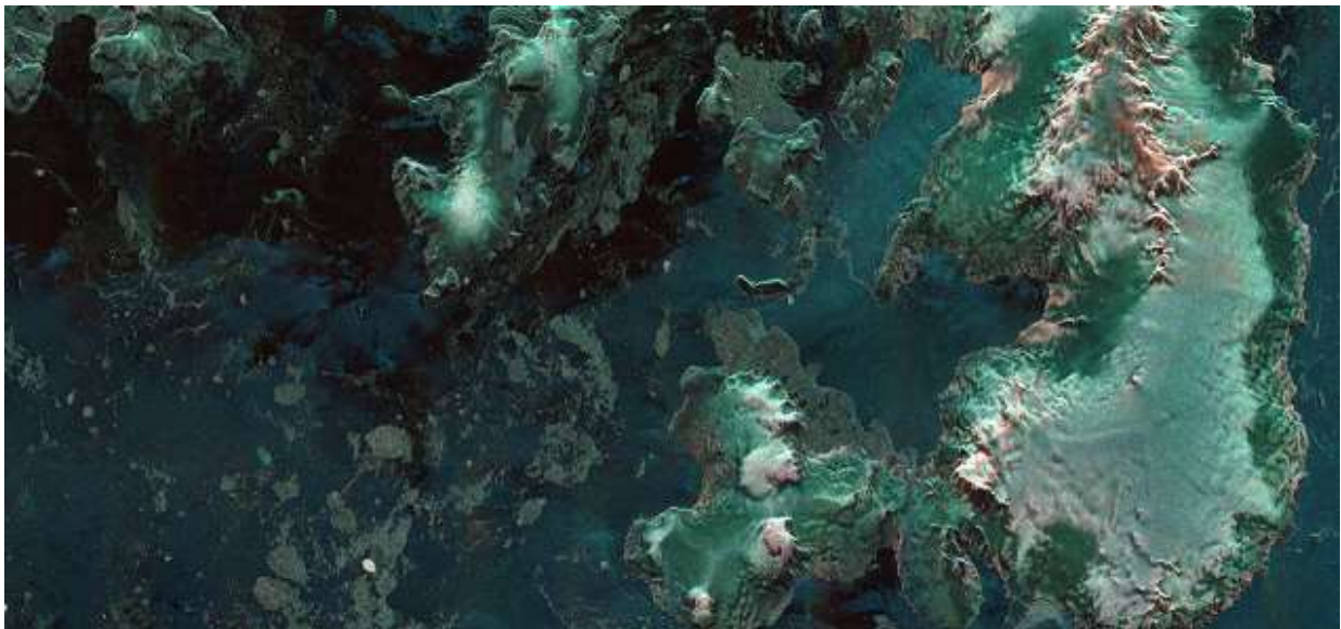
Figure 15: Duse Bay and Antarctic Sea ice 30m resolution Alt-Pol scanSAR (HH green, VV blue, HV red)
