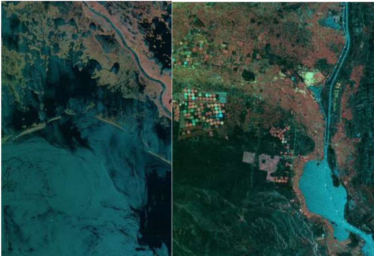
Figure 10: NovaSAR multi-polar images Mississippi Delta and gulf of Mexico (left), Suez Canal and red Sea 30m resolution Alt-Pol scanSAR with HH green, VV blue, HV red (Right)
