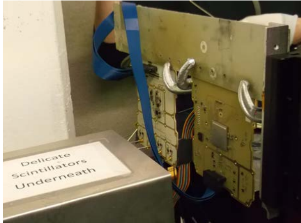
Figure 4 Two of the NRD electronics boards mounted on the 480 MeV proton irradiation beamline. The beam size was small to enable individual component irradiation. The Zynq can be seen in the middle of the board on the right hand side.
