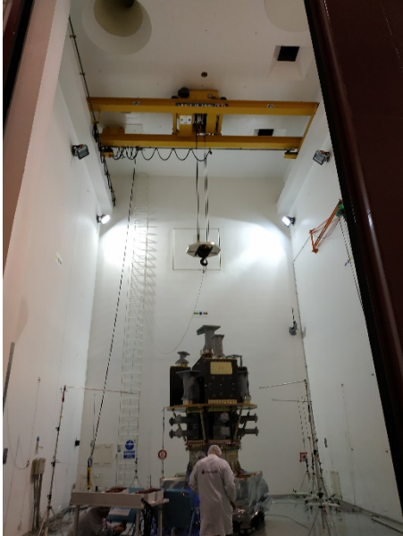
Flexi-3 PoC in Acoustic Chamber
