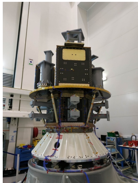
Flexi-3 PoC Vibration Tests Loaded
