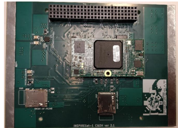
Figure 9: Command & Data Handling: Top view
