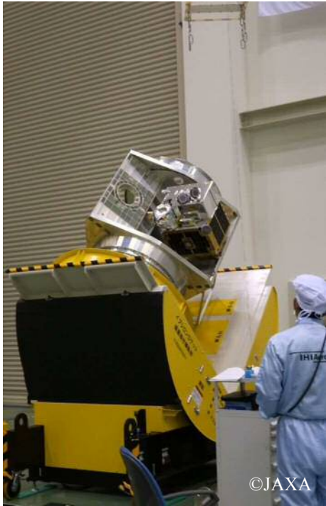
Figure 4: The rotating device used during fit-check of ALE-1
