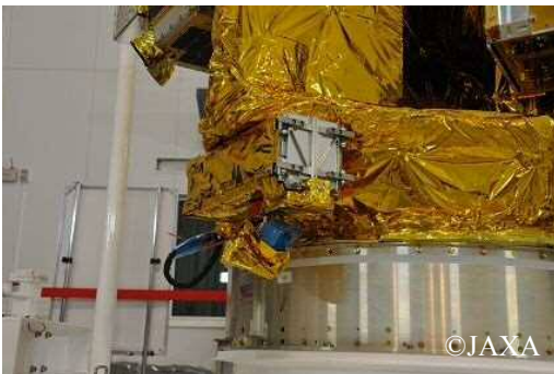
Figure 6: E-SSOD attached to ESMS with CubeSats stored inside
