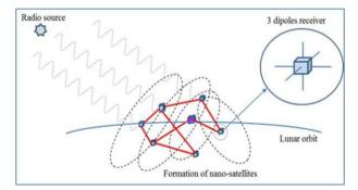
Figure 4: Satellite NOIRE network configuration
