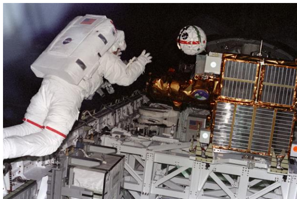
Figure 2: AERCam Sprint retrieval after a successful demo in the Space Shuttle cargo bay during STS-87. 6
