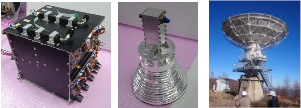
Fig.5 Left : High Speed X band Transmitter. Center : Medium Gain Antenna (MGA), Right : 10m Ground Station Antenna
