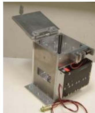
Figure 3: CubeSat XI-IV's separation mechanism
