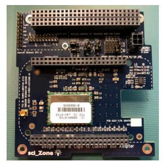
Figure 6: The LinkStar-STX3-PC104 Radio System.
