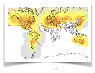
Figure 8: Approximate coverage area of the *LinkStar GSP-1720* duplex radio.
