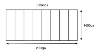
Figure 4: Push broom sensor showing the arrangement of 2 Mpx into 8 spectral bands.
