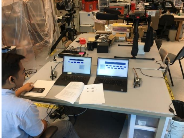
Figure 8: Lab set up with two E310 SDRs separated by a distance of 3ft with antennas at the Tx and Rx ports
